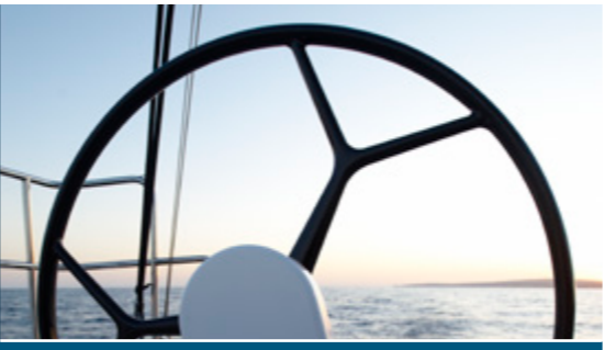
Double steering system, GRP wheels black, Y spoke, 2x900mm
