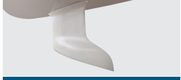
Shallow draft L-shape keel (1.37 m), cast iron
