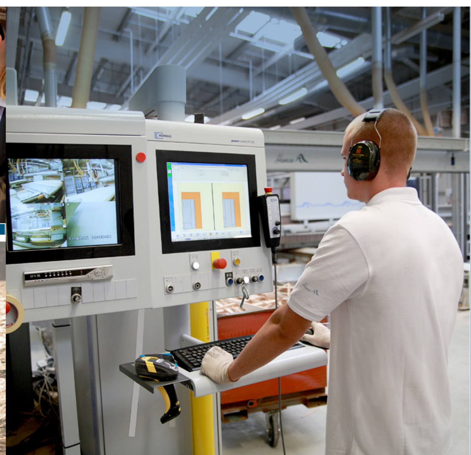
4 Before our carpenters build the interior of a HANSE 315, the wood panels are prefabricated using computer control.
